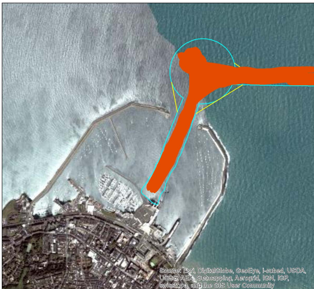
Figure 5-1: Combined Swept Paths of all of the Simulations with Proposed Channel Improvements
